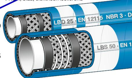
**'White band'** hose for all foodstuffs, milk, oils, fats, molasses, liquid chocolate and sirups. Temperature range -25°C to +90°C. The hoses can be temporarily steamed out with up to +130°C.
