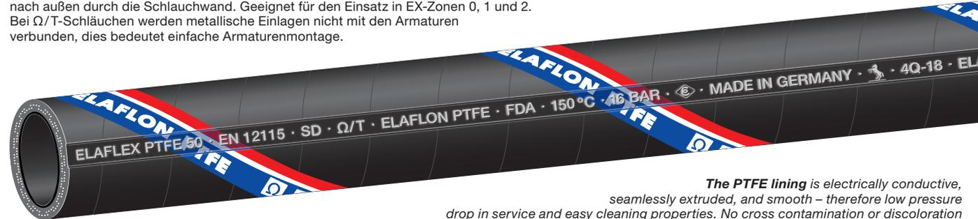
The PTFE lining is electrically conductive, seamlessly extruded, and smooth – therefore low pressure drop in service and easy cleaning properties. No cross contamination or discoloration of media thus being excellent when very pure media are being carried. Material conform to FDA / USP Class VI.
