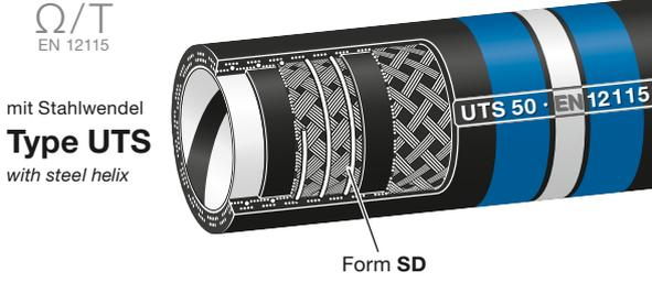
**Blue-white-blue universal tank hoses** for almost all liquid and pasty chemical and petroleum based products and solvents. Temperature range -40°C up to +100°C depending on medium. Steaming out for cleaning and sterilisation permissible up to +130°C for max. 30 minutes (open ends). Meets EN 12115, Ω/T.
