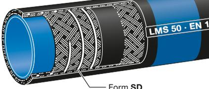
**Solvent hose** 'Blue Band' for most solvents, paints (also water based), water lacquer and dispersion, petroleum products, alcohols, aldehydes, esters and ketones. In short term operation also suitable for aromatic and chlorinated hydrocarbons. Further details see resistance chart. Temperature range -20° up to +80°C, short term up to +100°C. Open steam cleaning up to 130°C/max. 30 min.
