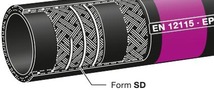
'Lilac Band' multi purpose hose for chemicals, acids (except for concentrated oxidising acids), alkalis, salt solutions, alcohols, polar solvents, acetates, aldehydes, ester, ketones, phenol, hot cooling water, hot air, **not** oily. Temperature range -40° up to +100°C (depending on medium). Open steam cleaning up to 150°C / max. 30 min.
