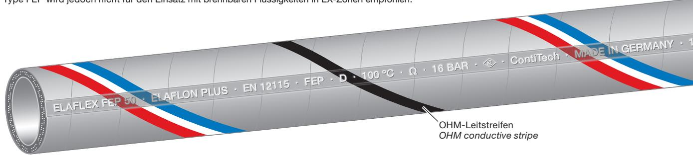
**Technical properties of the FEP lining:** Seamlessly extruded, smooth, therefore low pressure drop in service, easy cleaning properties. Excellent draining capability, no cross contamination or discoloration of media thus being excellent when very pure media is being carried. Materials conform to FDA and USP Class VI.
