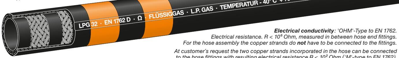
**Electrical conductivity:** 'OHM'-Type to EN 1762. Electrical resistance. R < 10<sup>6</sup> Ohm, measured in between hose end fittings. For the hose assembly the copper strands do **not** have to be connected to the fittings. At customer's request the two copper strands incorporated in the hose can be connected to the hose fittings with resulting electrical resistance R < 10<sup>2</sup> Ohm ('M'-type to EN 1762).
