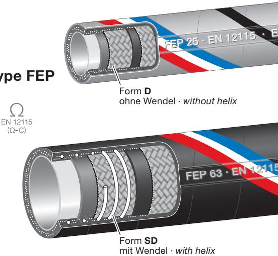
Universal hose **ELAFILON PLUS FEP** with seamless FEP lining, resistant to all commonly used chemicals, see resistance chart. Suitable for both suction and delivery (Type FEP D = delivery only). W.P. up to 16 bar, burst pressure > 64 bar. Temperature range from -30°C up to +100°C, briefly up to 130°C. Steaming out for cleaning and sterilisation permissible up to 150°C, max. 30 min (open system). Meets EN 12115.
