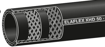
**Economy fuel oil reel hose without helix** for petroleum based products. Temperature range -30°C up to +70°C. Electrical conductivity < 10<sup>6</sup> Ohm.
