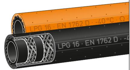
**Hoses for L.P. Gas dispensers.** Meet EN 1762 standard. For propane, butane and their mixtures. Highly flexible and long-lasting construction. Burst pressure > 100 bar. Temperature range **LPG 16 S** -30°C up to +70°C, **LPG 16** -40°C up to +70°C. DVGW and AS 1869 approved.
