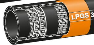
'Orange Band' **Liquefied Petroleum Gas** hose to EN 1762. For propane, butane and their mixtures to EN 589. Due to the very low permeability of the lining the hose is also suitable for natural gas (H<sub>2</sub>-content max. 5%). Due to the special design, these hose types do not need a pricked cover.
