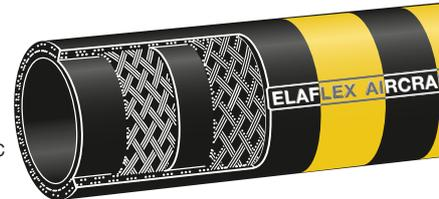
'Yellow Band' aircraft refuelling hoses, suitable for all aviation gasolines and jet fuels (JET A 1), deicing fluids and motor oils. Temperature range -30° up to +90° Celsius. Electrical resistance between 10<sup>3</sup> and 10<sup>6</sup> Ohm.
